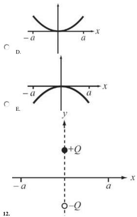
An electric dipole, a pair of equal but opposite charges. Two isolated point charges are fixed in the positions shown on the y axis; the positive charge is located at the point (0, b) and the negative charge is located at the point (0, -b). If a negative charge, -q, were moved along the x axis from x = -a to x = a, which graph best depicts the magnitude of the electric force it would feel during this motion?
