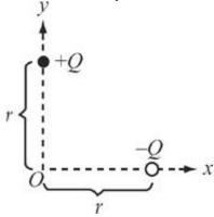
Two equal but opposite point charges are fixed in position on the x and y axes, as shown in the figure above. Which of the following arrows best illustrates the direction of the resulting electric field at the origin, O?
