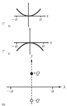
An electric dipole, a pair of equal but opposite charges. Two isolated point charges are fixed in the positions shown on the y axis; the positive charge is located at the point (0, b) and the negative charge is located at the point (0, -b). Which graph best illustrates the electric potential along the x axis, from x = -a to x = a?
