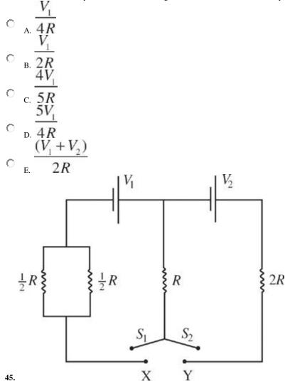
The circuit shown contains two switches:  $S_1$ , which can connect to point X, and  $S_2$ , which can connect to point Y. If both switches are left in the positions shown in the diagram, what is the current through the resistor R?
