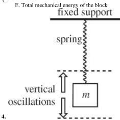
A block of mass m undergoing simple harmonic motion. Frictional forces are negligible and can be ignored. The maximum speed of the block is proportional to what quantity?
