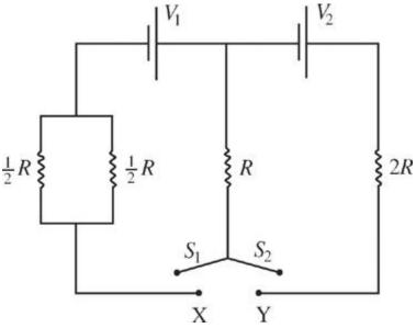
The circuit shown contains two switches:  $S_1$ , which can connect to point X, and  $S_2$ , which can connect to point Y. If switch  $S_1$  is left in the position shown in the figure but switch  $S_2$  is connected to point Y, what is the current through the resistor R?
