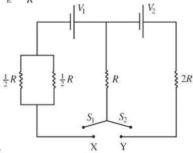
The circuit shown contains two switches:  $S_1$ , which can connect to point X, and  $S_2$ , which can connect to point Y. If switch  $S_2$  is left in the position shown in the diagram, but switch  $S_1$  is connected to point X, what is the current through the resistor R?
