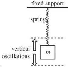
A block of mass m undergoing simple harmonic motion. Frictional forces are negligible and can be ignored. Which quantity would always be greater if the block oscillated with a smaller force constant?
