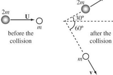
An object of mass 2m moving with velocity **U** strikes an object of mass m initially at rest. After the collision, the objects move away with velocities **u** and **v**, as shown.
