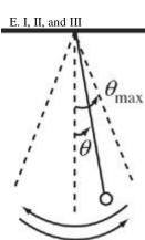
A simple pendulum, composed of a bob of mass m connected to the end of a massless rod, executes simple harmonic motion as it swings through small angles of oscillation. The largest angle the pendulum makes with the vertical is denoted by  $\theta_{\text{max}}$ . Frictional effects are negligible and can be ignored, and the pendulum is near the surface of the earth, where  $g = 9.8 \text{ m/s}^2$ . Which one of the following statements is true?
