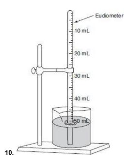
In this setup, a clean strip of magnesium with a mass of 0.040 g was introduced into the bottom of the tube, which contained a dilute solution of HCl, and allowed to react completely. The hydrogen gas formed was collected and the following data recorded:
