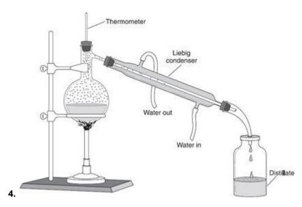
If the liquid being distilled contains dissolved ammonia gas, where will it be bound after distillation is completed?
