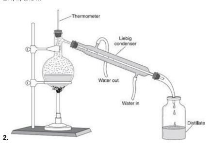
In this laboratory setup for distillation, where does the vaporization take place?
